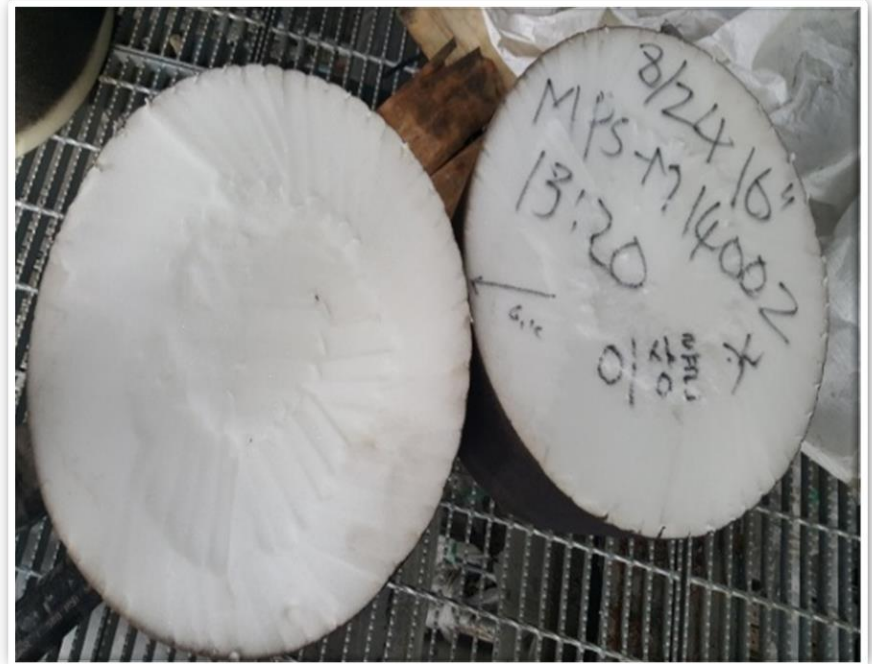
Sponge Pig Inspection
